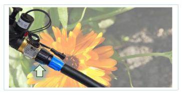
4. Connect "Threaded coupling or GA reducer" to Flow Sensor & attach 16mm
